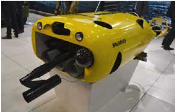
SAAB's Multi-Shot Mine Neutralisation System (MuMNS) ROV incorporating 3 disposal charges.
