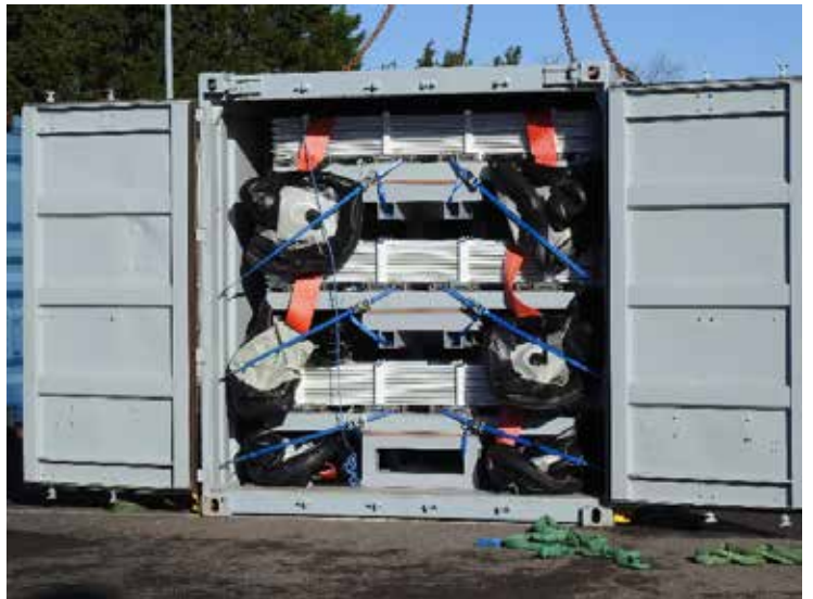
MHC is portable - three CABs stowed in 20' ISO ready for transportation
