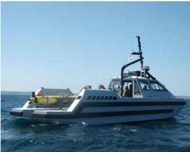
MASTT's RNL HAZARD undertaking UUV autonomous M500 ROV launch and recovery trials using Remus 600.
