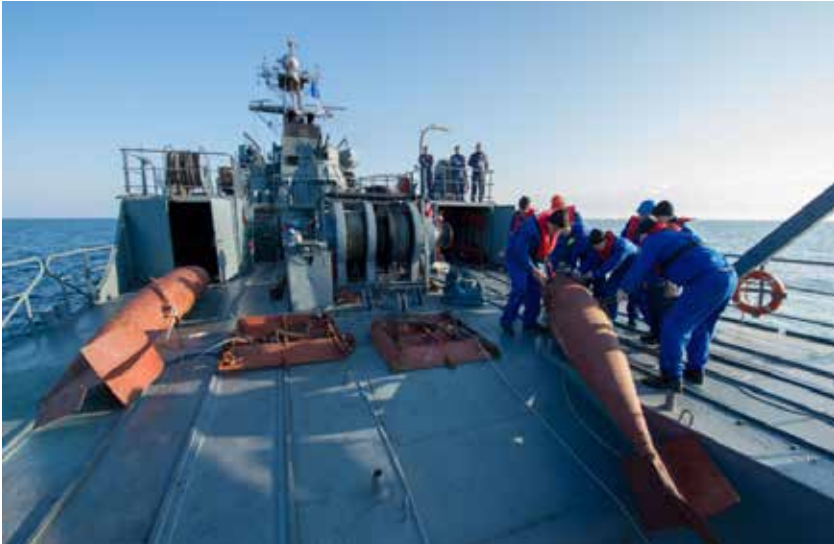
Romanian Ship Lt LUPU DINESCU conducts double oropesa mechanical sweep (those were the days!) in the Black Sea. Note the absence of cranes onboard the ex-Russian MHC.
