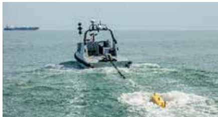
THALES workboat deploying T-SAM Synthetic Aperture Sonar (SAS) during trials.
