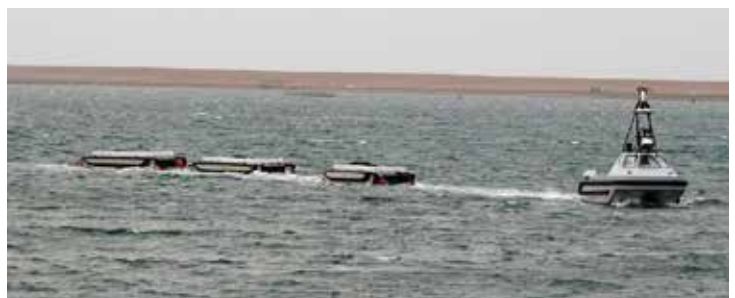
Atlas Elektronik's USV SWEEP Demonstrator under trials at Portland Harbour. (Note the 3 magnetic influence 'Coil Auxiliary Boats' (CABS) towed astern of the USV).
