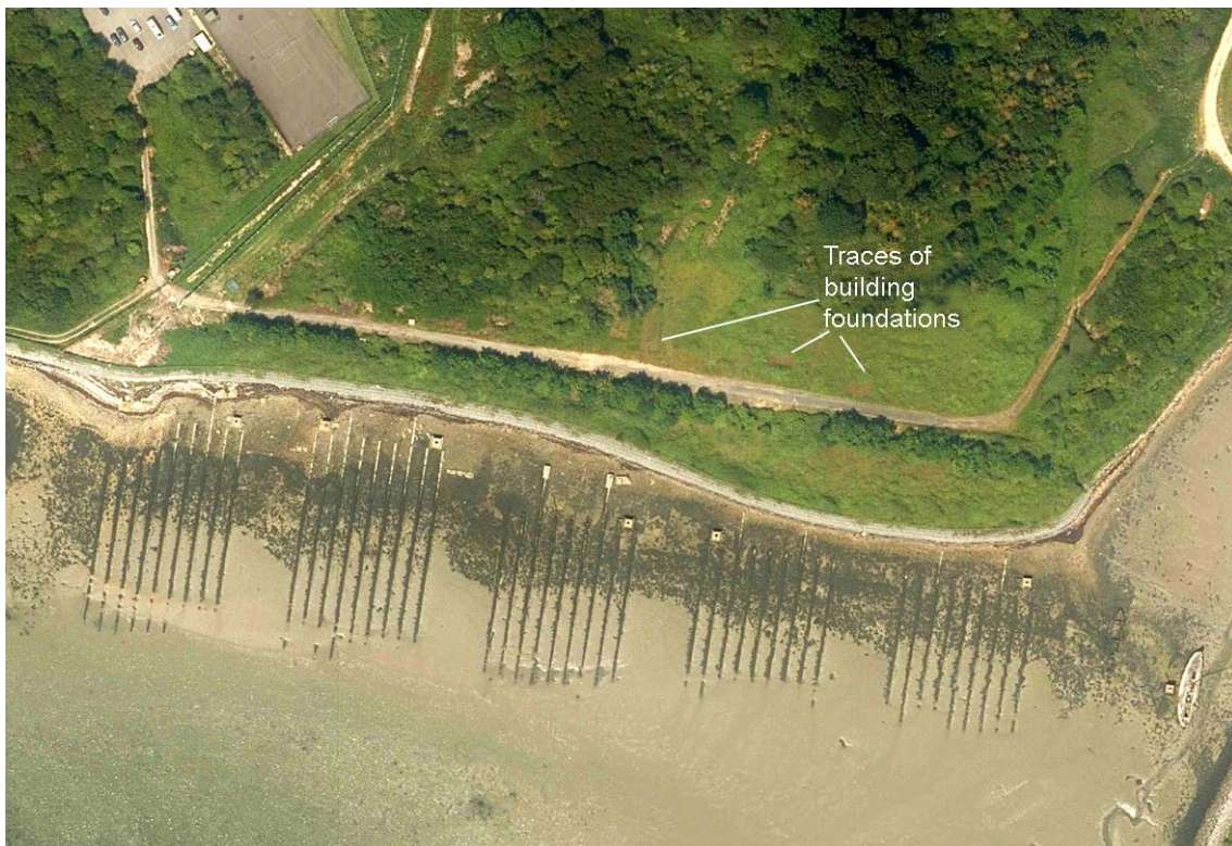
Figure 16: Extract of APGB mosaic aerial photographs taken in 2017 showing the slipways partially covered by silt and the sites of former Second World War buildings above the beach. 21-JUN-2017 ©Bluesky International/Getmapping.
