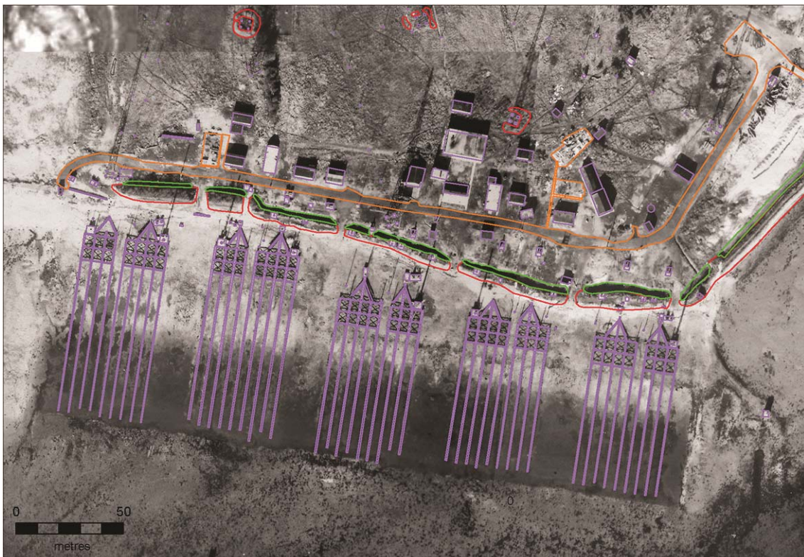
Figure 9: Aerial photograph overlain with mapping of key features of the slipways. Also see Fig 12 for detail. Purple = structure, red = bank, green = ditch and orange = extent of feature. Extract of RAF aerial photograph RAF/106G/UK/955/RVp3/6246 30-OCT-1945. Historic England Archive RAF photography.
