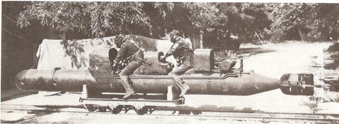
'Maiale'pig, Italian human torpedo that carried two frogmen and a war-head bomb of five hundred pounds of high explosive. Dry land practice.
