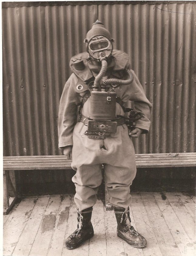
'Port' Party diving suit with self contained breathing apparatus (Nitrogen/Oxygen) specially developed for D-Day operations. All non-magnetic.
