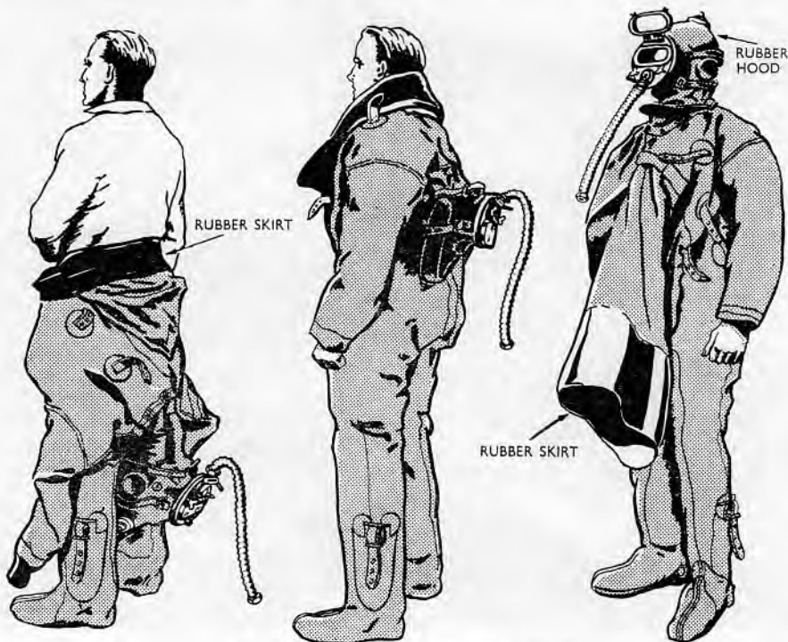
A.S.W.D.D.—First three stages of dressing
