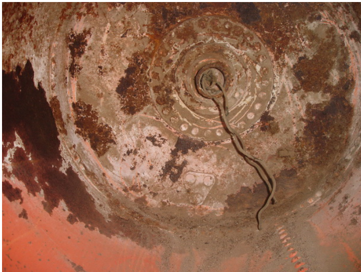
Interior base, showing wires which entered the body of the mine through a sealed gland, attached to the base exterior. The original red lead internal paint is largely intact. A total of around 300 rivets were used in the mine's construction.
