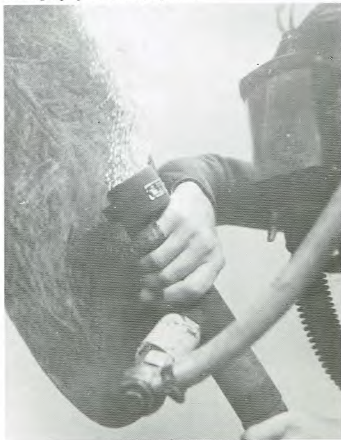
Dressing a propellor with u/w grinder.
