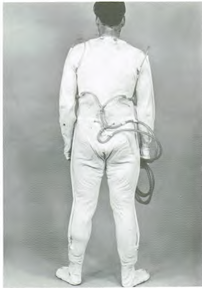
Closed circuit water heated suit. Heat is controlled by varying the water flow.
