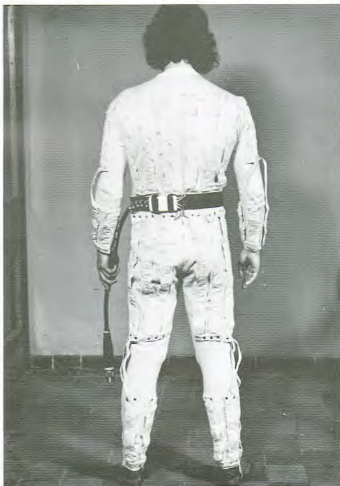
Electric heated suit capable of supplying up to 1.2 kw at 28 v DC.
